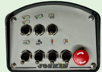
Control box with several functions adapted to each machine
