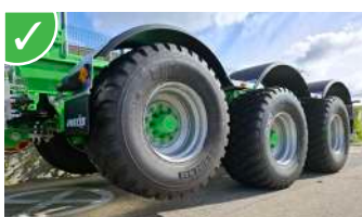
Front lifting axle (up to 150 mm high on triple-axle models) to limit wear on the road and increase the load on the tractor when needed.
