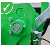
Drawbar with silentblock suspension (D10 and D14 models).
