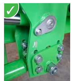
Adjustment of the steering angles on steering axles according to the size of the wheels and the road width allowed by CE standards.
