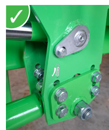
Adjustment of the steering angles on steering axles according to the size of the wheels and the road width allowed by CE standards.
