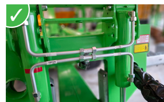
Numerous rigid pipes for clean installation and better oil circulation.
