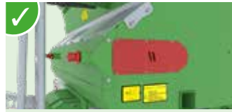
✓ Mechanical moving floor tensioner (using traction).
