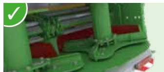
✓ HARDOX protection wear plates.
