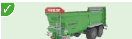
✓ Openwork 450 mm front extension in galvanised steel.
