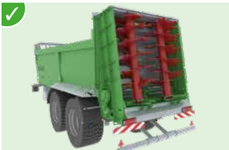
✓ 2 vertical Ø 1,010 mm beaters in continuous spirals on Ø 219 mm tube. Height of the spreading unit: 1,770 mm (series 11), 2,220 mm (series 14) Clearance height under guillotine door: 1,355 mm (series 11), 1,700 mm (series 14).
