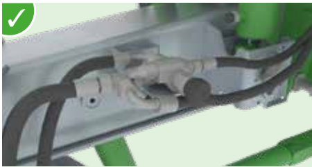
✓ Pressure regulator with compensated pressure for moving floor speed.
