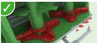
✓ 2 star-shaped spreading discs with 4 blades.
