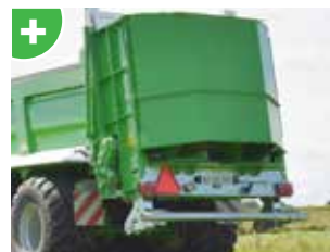
Canopy with quick coupling system (for vertical beaters)
