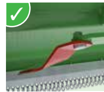
195mm self-retractable blades with twisted profile: better crankcase ventilation and more uniform distribution (on TR-ATR-TRT-BEV).
