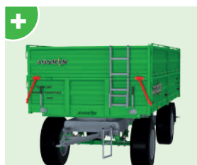
Front return springs for easy handling of the drop sides (only on models 4525 and 5025).
