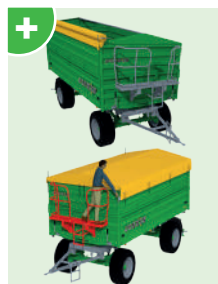
Manual roll-up cover + platform for optimal safety
