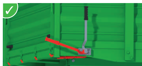
Adjustable locking system with a very large number of hooks on the side and rear drop sides to ensure a correct pressure on the seals.
