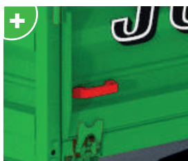
2 handling handles on each basic drop side.
