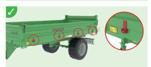
4 simplified, self-tightening high tensile steel drop side hinges for a sturdy base and perfect watertightness.
