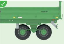
**Roll-Over bogie with** bolted table on doubleaxle models (wheels: max. Ø 945 mm). Optional on bogie: braking power in proportion to the load (air brakes compulsory).
