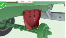
Movable, bolted running gear. Adjustable in height (to fit large wheels) and depth (to adjust weight on tractor on single-axle trailer).
