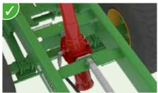
Telescopic tipping cylinder on a double-oscillating frame with greased bearings.
