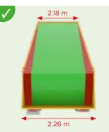
Tapered body (2.18 m at the front and 2.26 m at the rear) to facilitate unloading.
