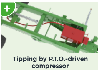
59.6° tipping system with telescopic cylinder on a double oscillating frame placed in an advanced position in the chassis.
