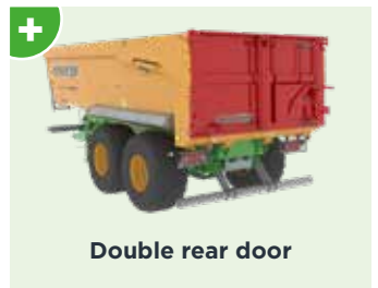
1-part hydraulic door with cylinders protected under the arms.
