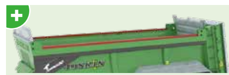
✓ 70 x 70 mm PVC protection of the upper body edges.
