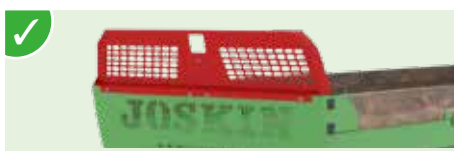
✓ Openwork front extension in galvanised steel
