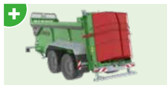
✓ Double canopy with hydraulic boards for field edges and safety on the road.
