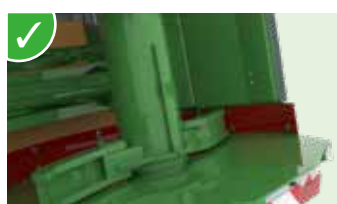
✓ HARDOX protection wear plate .
