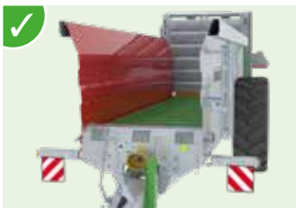
✓ Narrow body made of 4 mm sheet metal (S420MC) with reinforcement folds over the entire length.
