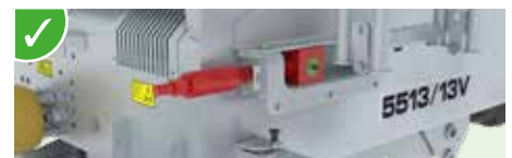
✓ Mechanical chain tensioners with tension springs and visual adjustment indicator.
