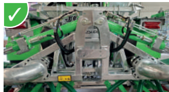
2 cylinders for folding the boom in working position with check valve and solenoid valve.
