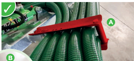
(A) Injection hoses with adjustable locking to protect them from wear due to vibration. (B) Flexible, rounded collar to hold and protect the hoses.
