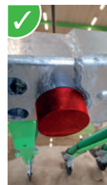
Silentblock for the last folded part to prevent friction and vibration.
