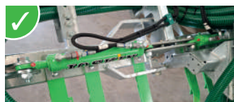
2 floating cylinders on springs with check valve for each double folding system, for a good follow-up of the ground + rocker to limit space requirement.
