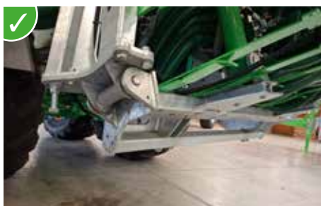
Inclined kinematics to transfer as much weight as possible to the slurry tanker during travel.
