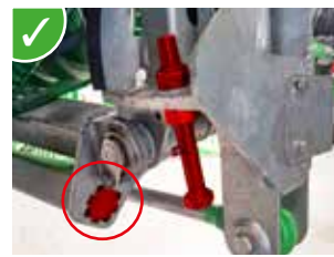
Adjustable stop to ensure even pressure of all elements on the ground.
