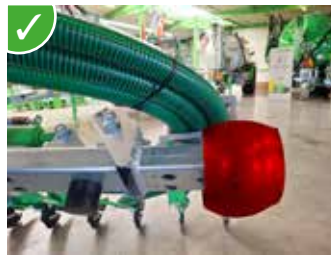
Anti-crash safety at the end of the boom with protective cap
