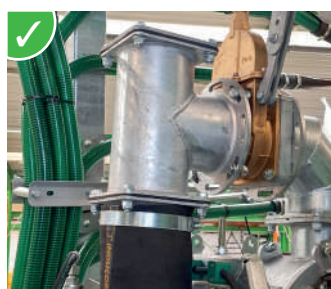
Macerator feeding valve (Ø 150 mm) with extra outlet for optional exact scatterer.
