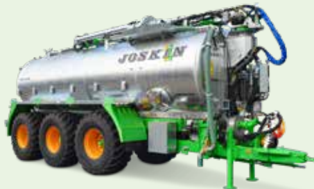
Euroliner Triple-axle tanker with large volume on independent chassis
