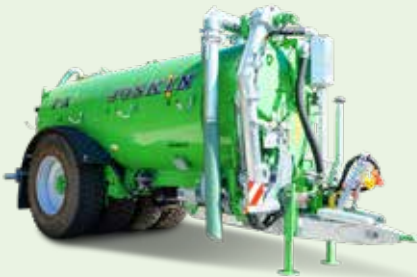
Tetrax2 4 large wheels in a row to avoid ground compaction
