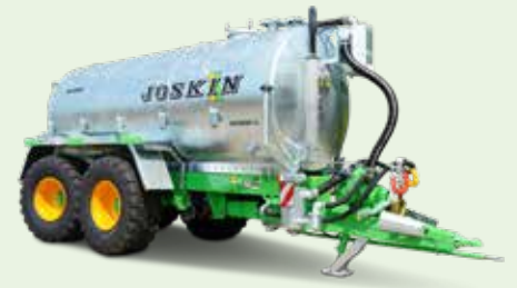
Quadra Double-axle tanker with large volume on independent chassis
