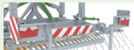
LED lighting with striped boards (red and white).
