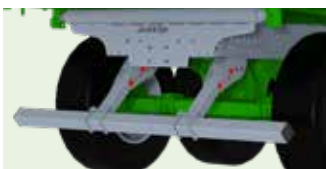
Multiposition rear bumper with height adjustment (Delta models).
