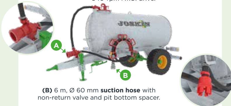
(A) Centrifugal filling pump: 1,000 l/min flow, 540-rpm P.T.O. drive.
