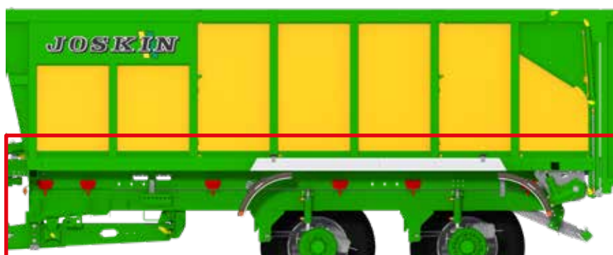
2 independent tubular chassis with 2x6 fasteners for a perfect strength.
