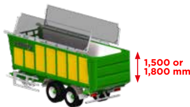
DUO-COVER (2 covering nets on frame, specific for silage) , only with extensions A B C D .
