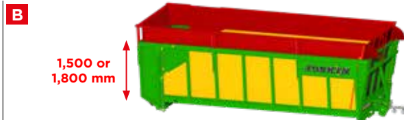
Individually retractable hydraulic side extensions from 50 to 550 mm - manually folding front extension - 4-position mechanical rear part.
