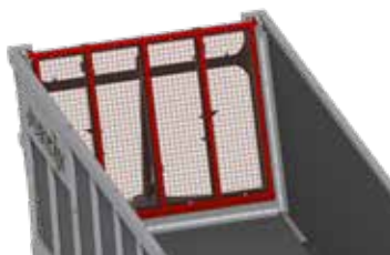
Beet grate to protect the transparent front wall from dirt.
