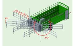
270° pivoting fold-back fences with rear (against door) or side storage, expendable from 2.27 m to 3.67 m.
