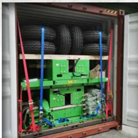
6x Trans-EX 5 t tipping trailer and 4x 3 t tipping trailer in one single 40ft HC container
